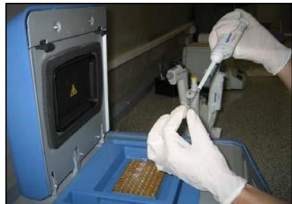
Grinding leaf samples with a tissue homogenizer
